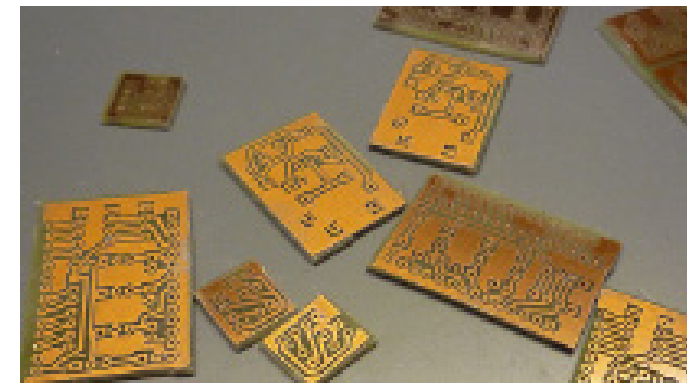
3.3.3 Fritzing used in production: All above images show the process of making custom PCBs for Goldsmiths University's home sensor network research project.
