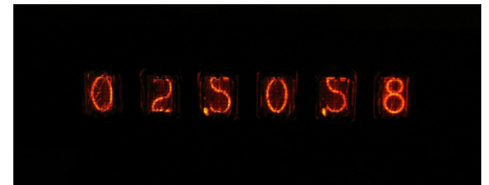
3.3.1 Hobby practitioner arms22 using Fritzing, a microcontroller and extra bits to find a contemporary way of using old Nixie Tubes. Top to bottom: 1. Fritzing breadboard view, 2. microcontroller, Fritzing generated custom PCB and Nixie Tubes in self made box 3. Nixie Tubes displaying numbers
