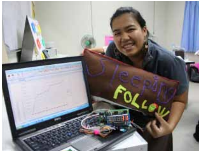
3.2.1 Sleeping tracker project using a GoGo board. Five switches hidden underneath the pillow detect when your head moves.
