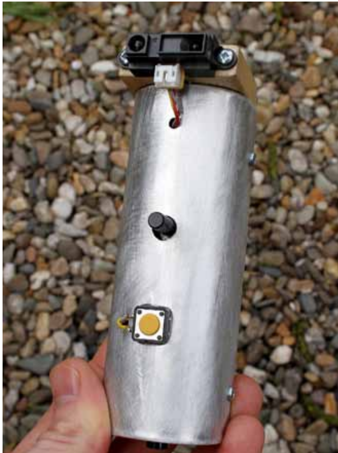
3.3.2 Gijs Gieskes' Wave Table Radar is an experimental contemporary re-creation of a theremin. Picture on top without, above with case. For purchase.
