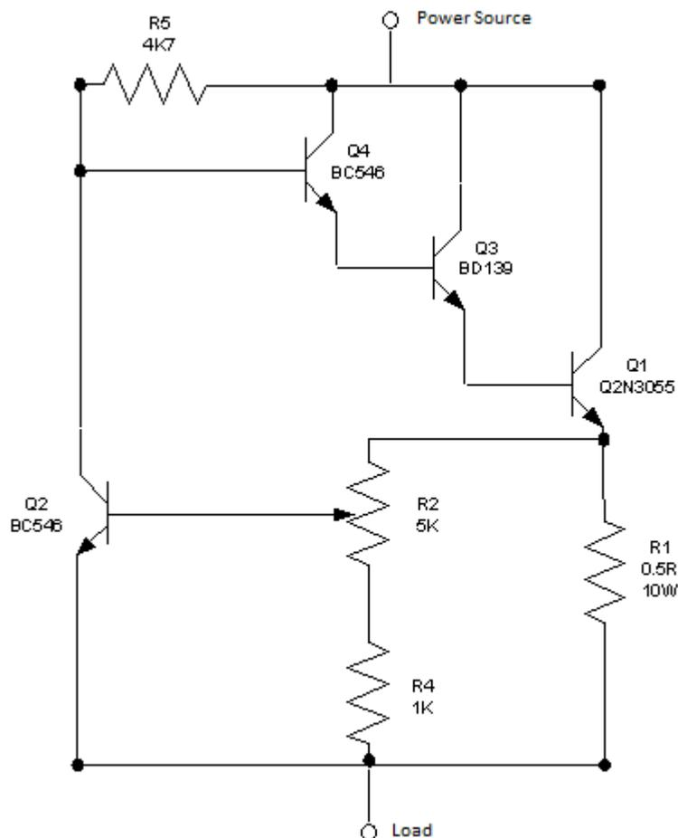
R1 is the current sense resistor. When R2 potentiometer is at minimum resistance (the center tap connected to R1), and the current drawn by the load reaches 1.2A the voltage across R1 will reach 0.6V and Q2 begins to conduct current and shorts the base voltage of Q4 to ground. The shorting of Q4 base to ground reduces the base current and the output voltage sensed by the load, preventing the current from flowing further.
